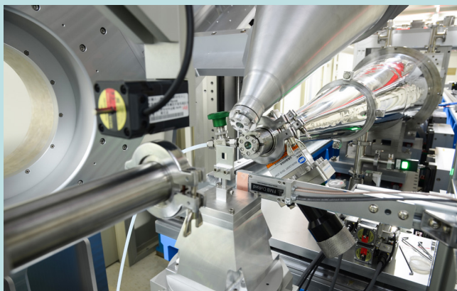
Fig. 2: Both the Bragg grommetry and small q range detection systems are centered to the sample.
